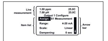
**FIGURE 4-2. Programming Screen Showing Item List.** The position of the cursor is shown in reverse video. See Section 4.2 and 4.3 for more information.
